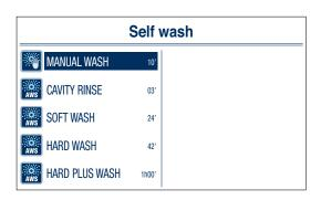
Select the desired type of washing cycle directly on the touch screen or turn the Scroller+ to the type of washing desired and confirm by pressing the Scroller+.
