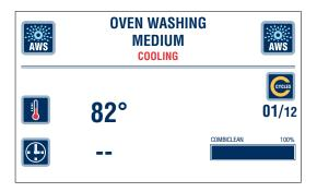
• The display shows "COOLING" if the oven temperature is high or "WAIT" if the oven temperature is too low.
