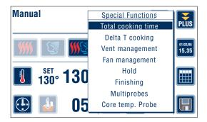
Select "Delta T" directly on the touch screen or turn the Scroller+ to "Delta T" and then confirm by pressing the Scroller+.
