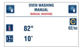
• The oven proceeds with the subsequent cycles, the display shows the time remaining until the end of the washing cycle (total duration of wash: 10').
