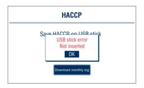
If the USB pen is not inserted, a window will appear signalling the problem.
