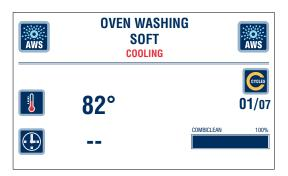
• The display shows "COOLING" if the oven temperature is too high or "WAIT" if the oven temperature is too low.
