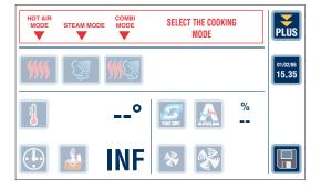
Select the cooking mode (Convection, Steam or Combined) directly on the touch screen by pressing the symbol below the description of the type of cooking.
