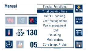
Select "Fan management" directly on the touch screen or turn the Scroller+ to "Fan management" and confirm by pressing the Scroller+.
