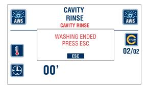
The oven proceeds with the subsequent cycles, the display shows the time remaining until the end of the washing cycle (total duration of rinsing: 3').
