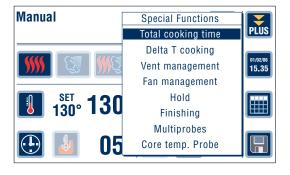
Select "Multiprobes" directly on the touch-screen, or rotate the Scroller+ until you are positioned on "Multiprobes" and then confirm by pressing the Scroller+.
