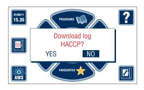
With the first start-up of the day, the oven prompts the operator to save the HACCP Log on a USB pen.
