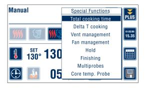
Select the desired function directly on the touch screen or by turning the Scroller+ to the desired function, then confirm by pressing the Scroller+.
