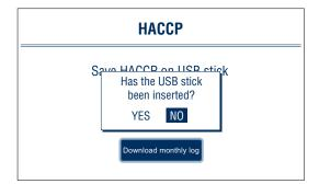
A screen will appear asking the operator to insert a USB pen.
